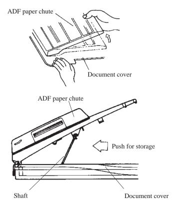
Figure 4.3 ADF paper chute setting
